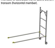
**Step 3** Lock brakes on castors of second doorbase frame and attach horizontal braces to **INSIDE** of standards.
