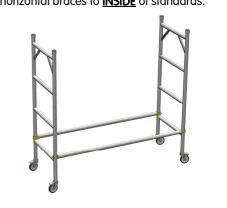
**Step 4** Install diagonal brace (silver) from bottom transom, to third transom up (2 spaces). The brace should be as close as practical to the outside.
