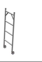
**Step 2** Attach 2 horizontal braces (yellow) to <u>INSIDE</u> of standards (vertical member) of doorbase frame above bottom transom (horizontal member).
