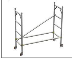
**Step 5** Install platform on the first or second rung as required.
